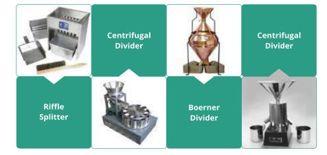
Riffle splitters can perform well, but the results rely on the skill and training of the operator. The sample needs to be fed into the riffle splitter.
