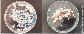
Fortified Rice turning blue Fortified Rice turning red on on reaction with ferricyanide reaction with KSCN indicating indicating presence of iron in Fortified Rice Kernel
